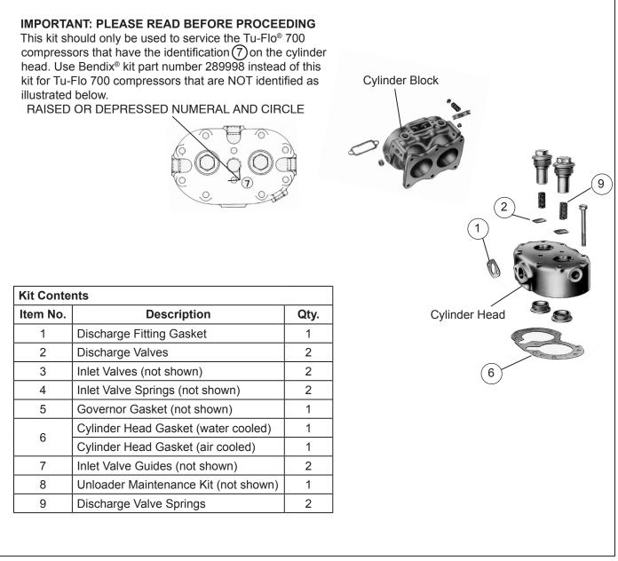
Figure 1 – Compressor Exploded View
